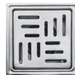
6311-10-80S1 Floor Drain SUS304 Size 102*102 mm Height 34 mm Seal Type Self Seal ABS Flow Rate \geq 15\text{L}/\text{Min} Outlet OD 42 mm Drain Core 6310-A0-8000
