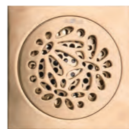
6310-60-80SK Floor Drain Brass Size 100*100 mm Height 35 mm Seal Type Self Seal Brass Flow Rate \geq 22\text{L}/\text{Min} Outlet OD 40 mm Drain Core 6310-A0-8000
