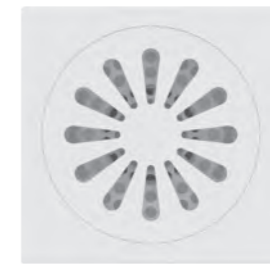
6303-61-80CW Floor Drain Brass Size 100*100 mm Height 43 mm Seal Type Self Seal Brass Flow Rate ≥15L/Min Outlet OD 40 mm Drain Core 0303-A1-7900
