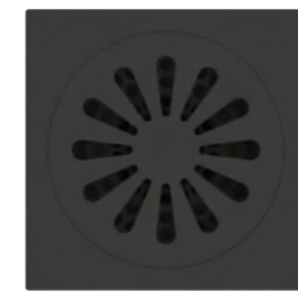
6303-61-80MA Floor Drain Brass Size 100*100 mm Height 43 mm Seal Type Self Seal Brass Flow Rate ≥15L/Min Outlet OD 40 mm Drain Core 0303-A1-7900
