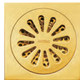
6303-61-80PK Floor Drain Brass Size 100*100 mm Height 43 mm Seal Type Self Seal Brass Flow Rate ≥15L/Min Outlet OD 40 mm Drain Core 0303-A1-7900
