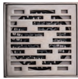
6310-10-80AB Floor Drain Brass Size 100*100 mm Height 35 mm Seal Type Self Seal Brass Flow Rate \geq 22\text{L}/\text{Min} Outlet OD 40 mm Drain Core 6310-A0-8000
